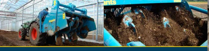
The deepspader series are standard with unique Imants spade shaft with left and right arms and interchangeable spade blades (SX). On the 60SX270DR, 65 and 70 series it is possible to have another spade shaft.
