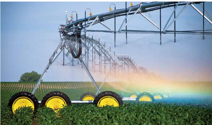
T-L’s flexible corner connection transfers the smooth, continuous movement of the pivot system to the corner arm.
