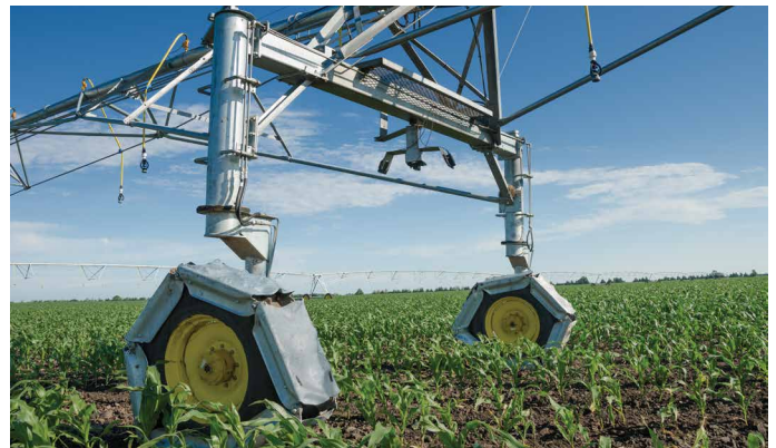
Hydraulic motors are coupled directly to the planetary wheel hub allowing a narrower travel profile for reduced crop loss.
